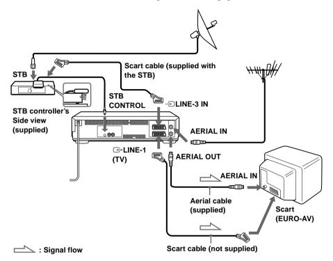
You can watch programmes from the Set-Top Box connected to this VCR on your TV even when the VCR is turned off using the Line Through function. When you turn on the STB, this VCR automatically sends the signal from the STB to the TV without turning itself on.
